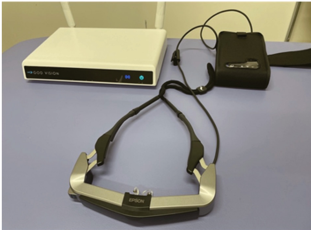
Fig. S1. Wearable glasses-type device Moverio BT-35E, and wireless imaging transmission system GV-200
